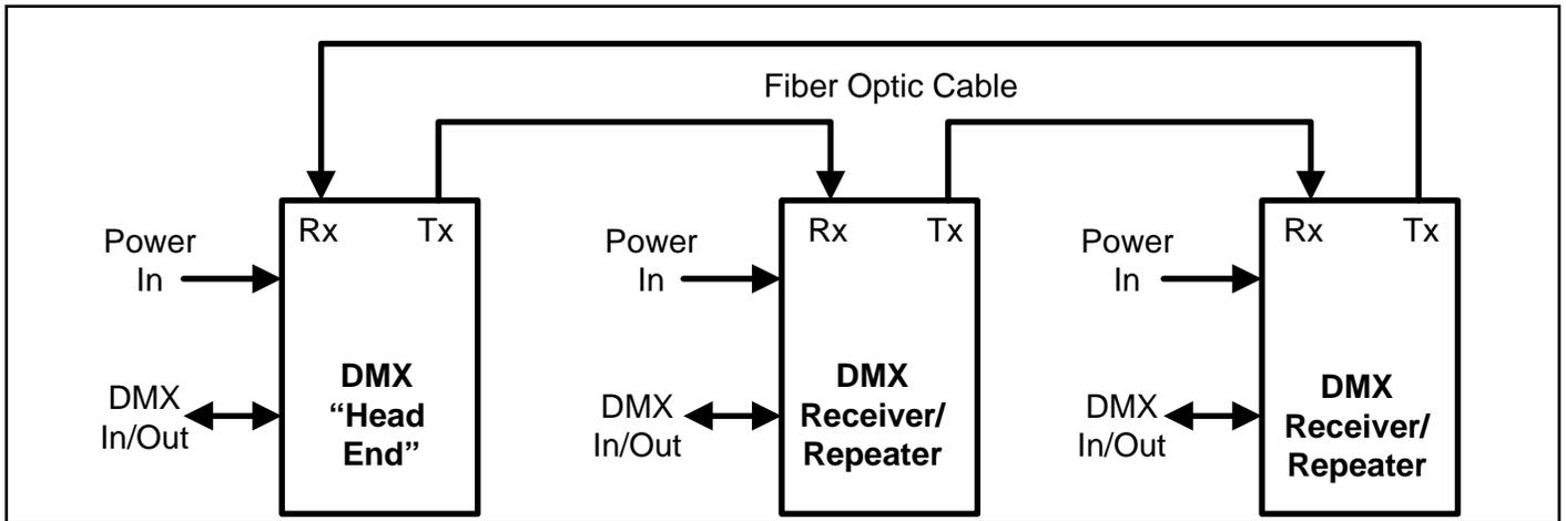
Figure 3, Typical DMX-512A/RDM fiber optic transmission system.
