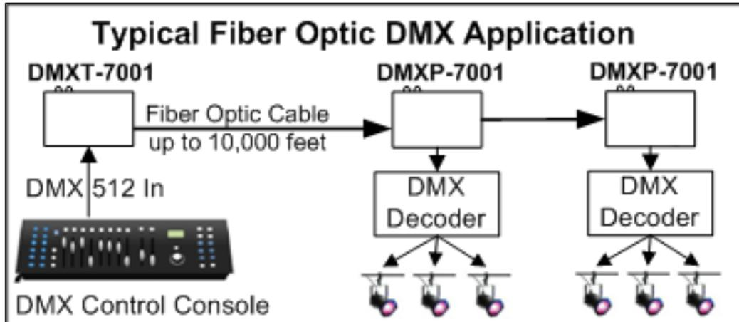
Figure 1, Typical DMX-512 fiber optic transmission system.
