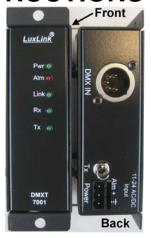
The DMXT-7001 and DMXP-7001 are designed to transmit, receive and repeat standard ANSI E1.11-2008 (DMX-512-A) signals at data rates from DC to 1Mb/s on a single optical fiber. The unit may be used for point-to-point or in drop and repeat applications.
